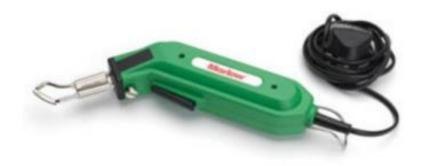
This industrial hot knife rope cutter is a hand operated tool that will cut and seal end on all synthetic cords and ropes. It takes a mere 6-8 seconds to heat up to approx 600°C it will melt the rope and seal the ends. Heat may be controlled by switching tool on and off.
